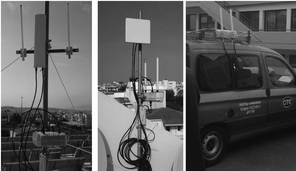
Fig. 14. MRBS Antenna, transceiver, GPS-RS system-MS.
